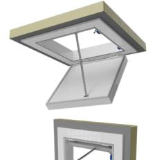
Motorized flaps for smoke evacuation in case of fire. Specially designed to be installed in cold or even frozen chambers with excellent thermal and sealing performance. Homologation of mechanical smoke extractor accessory according to standard EN-12101-3, with F400 and F300 certification.
