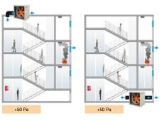
systems with standby fan and test certificate according to the European standard
